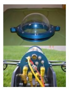
water. The ability to attach and detach these connectors rapidly without disrupting the watertight seal adds to Barracuda's modularity. The end caps are pulled together on the longitudinal axis of the hull by turnbuckles and threaded rods. The use of turnbuckles instead of latches alleviates much of the torsional stress on the sidewall of the main tube that could be caused by closing the latches.
