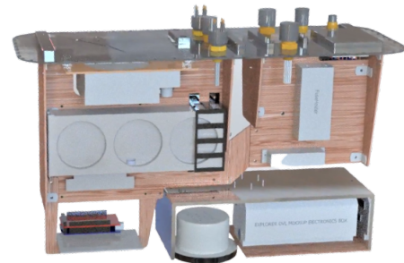
Fig. 3. Compared to Marlin’s rack, Nemo’s new vertical rack design allows for easier accessibility to components for electrical members.
