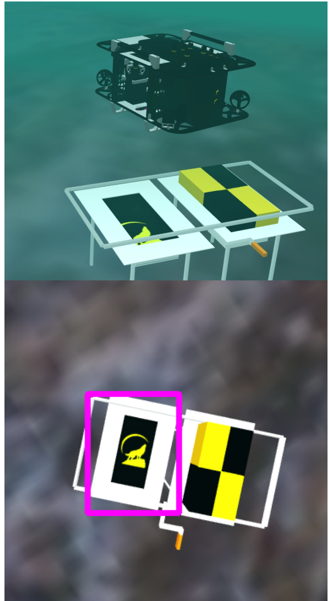
Fig. 7. Nemo utilizes its vision system to continuously readjust and align itself to the bin in the simulator.
